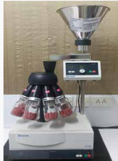
Automatic Seed sample divider
